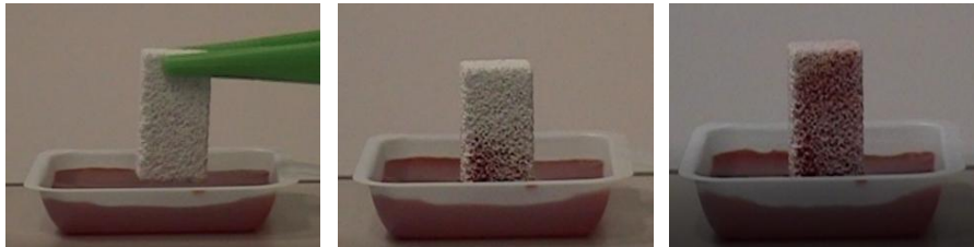
Figure 4 – The interconnected micro/macro-porous structure of hydroxyapatite enables fluid absorption.
